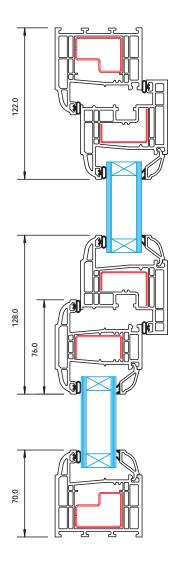
Internally Glazed Ovolo Outer Frame: B07 Sash: B38 Transom: B22 Bead: B60
