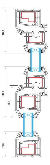
Internally Glazed Bevelled Outer Frame: B03 Sash: B33 Transom: B16 Bead: B50
