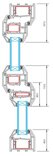
Externally Glazed Outer Frame: B02 Sash: B31 Transom: B10 Bead: B50
